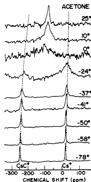
Figure 7. Cesium-133 NMR spectra at various temperatures for a mixture of 0.02 M CsTPB and 0.01 M cryptand-2.2.2 in acetone. The dashed lines give the positions of the Cs^+ \cdot C222 complex and the Cs^+ ion at the corresponding temperatures.
